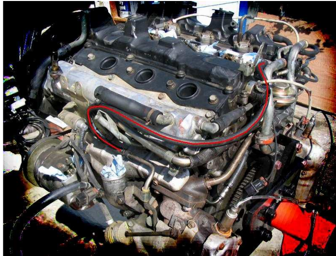
Figure 12: 6mm Hose in Place
