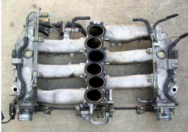
Figure 8: Bottom Side of Plenum with Hoses
