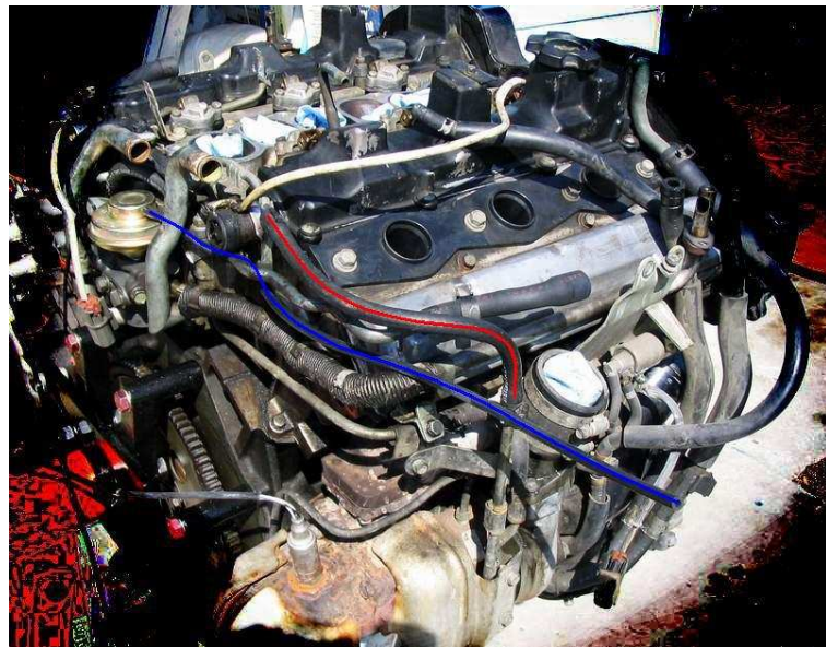
Figure 15: 6mm Hose and 4mm Hose in Place
